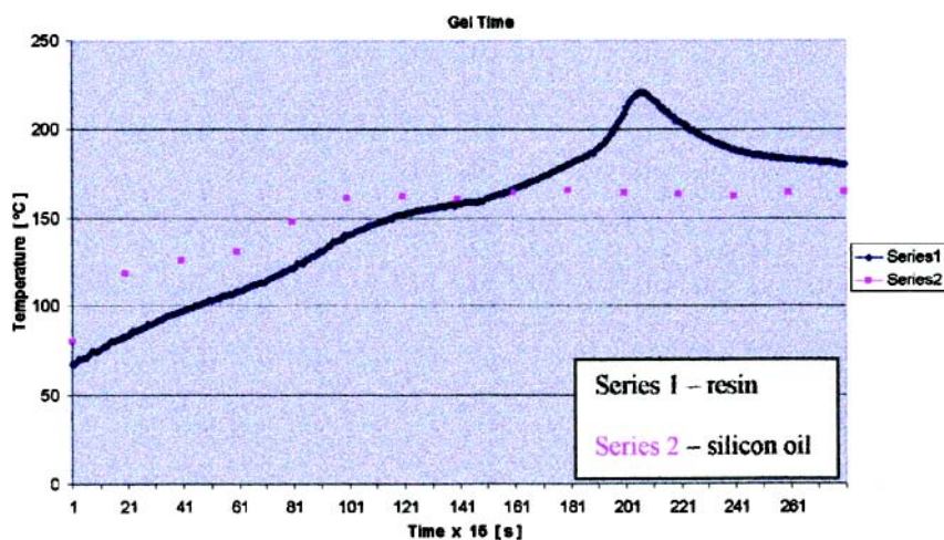
FIGURE 1 Variation of the resin temperature in the gel time (RTM 6.).
